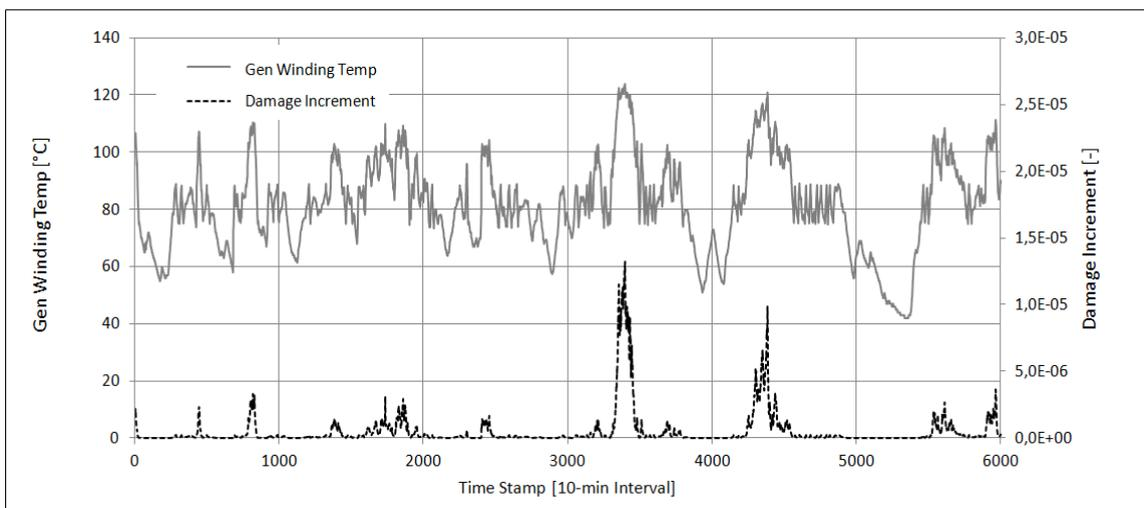
Figure 7: Damage calculation: thermal aging of generator winding insulation
