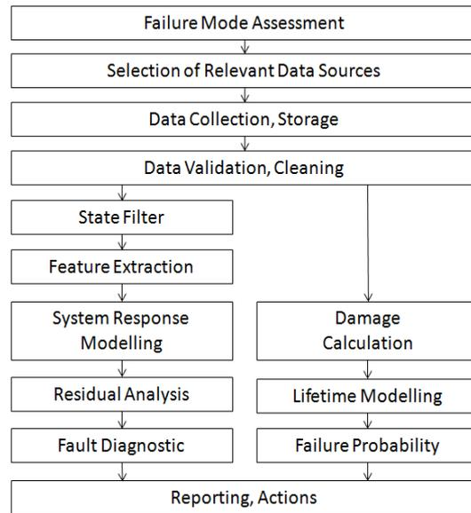
Figure 1: Overall workflow, diagnostics & prognostics with SCADA logs.
