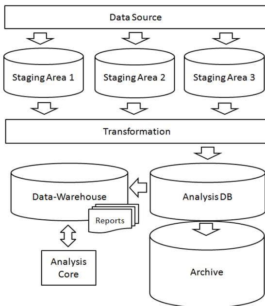
Figure 2: SCADA Database architecture as platform for wind turbine performance and condition monitoring.
