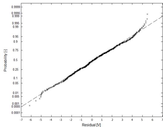
Figure 6: response model quality testing using a normal probability plot.
