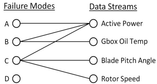
Figure 3: Correlation between failure modes and available data streams.
