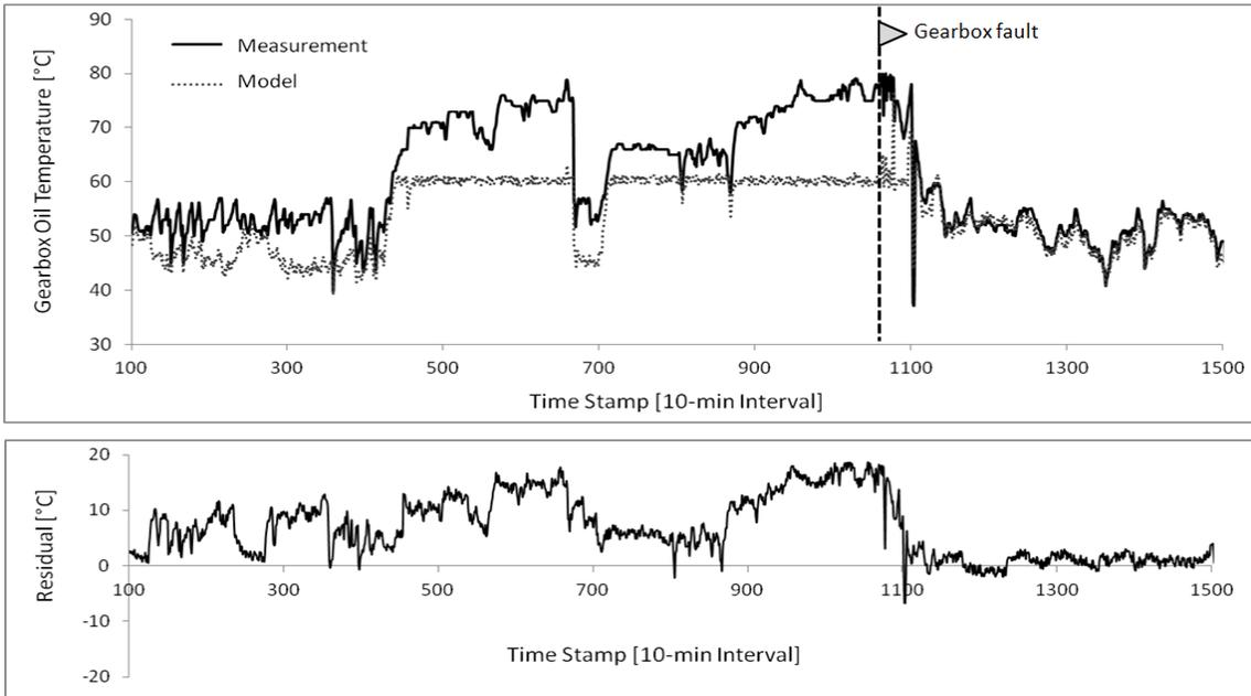
Figure 5: System response modelling of gearbox oil temperature, residual value deviation as fault indicator
