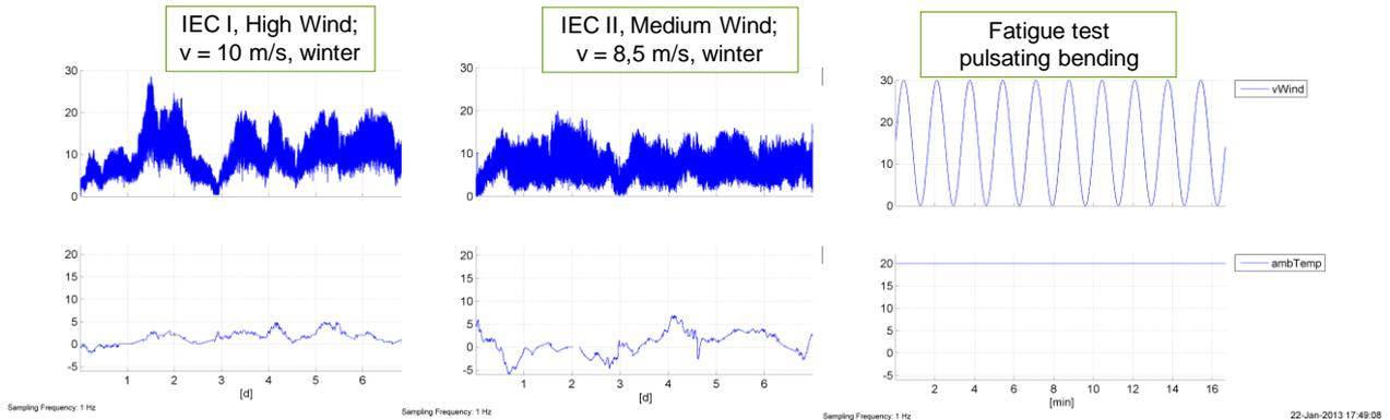
Fig. 6: Wind speed time logs for high and medium wind class and a load cycle for a pulsating bending fatigue test.
