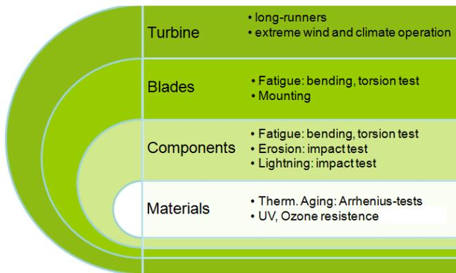
Fig. 4: Validation hierarchy for turbine blade as a result of component maturity demonstration approach
