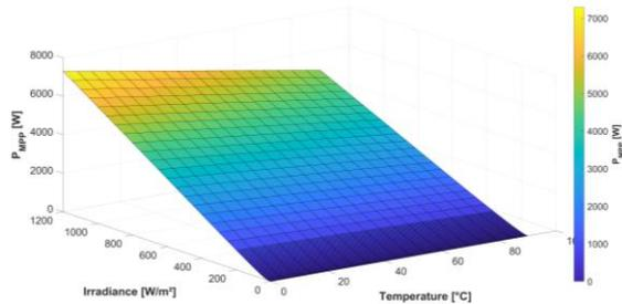
Figure 2: Characteristic diagram  $P_{MPP} f(T,G)$
