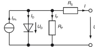
**Figure 1: One-diode model of a PV cell [13]**
