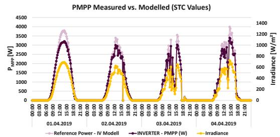
Figure 4: Measured vs. modelled string power
